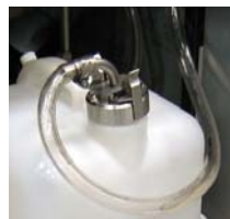
Automatic oil level top-off feature
