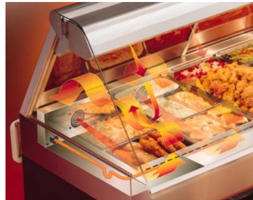
Fig 3. Henny Penny's Thermo-Vec display heating technology produces precise, even heat without hot or cold spots and fogged glass. Food is warmed evenly by thermostat controlled heat from electrical elements below and radiant heat from overhead. Low power fans gently circulate the air, continually dispersing moisture throughout the cabinet and away from the surface of the glass. Flow vents along the front and back allow the free movement of air. Special sensors detect and immediately compensate for changes in air temperature during serving.
