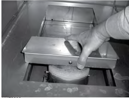
Figure 3-4 Removing Concentration Ring Assembly
