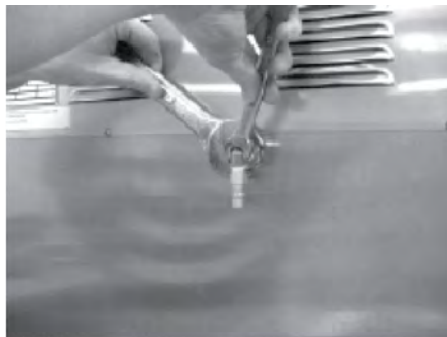
Figure 2-1 Tightening Fitting Nut
